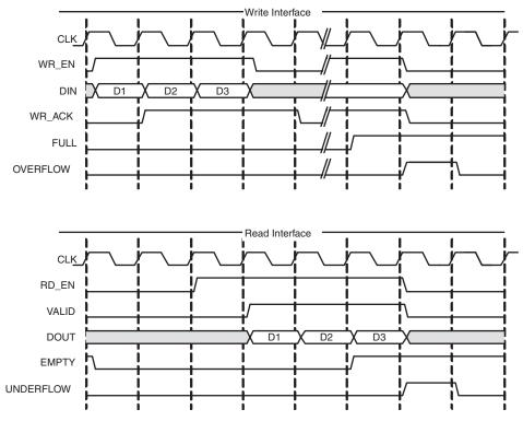
Figure 4-11: Handshaking Signals for a FIFO with Common Clocks
