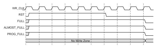
Figure 4-27: Block RAM, Distributed RAM, Shift RAM with Full Flags Reset Value of 1 for the Reset Pulse of More Than One Clock
