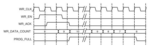
Figure 4-13: Programmable Full with Assert and Negate Thresholds: Assert Set to 10 and Negate Set to 7
