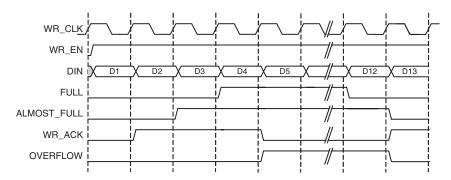
Figure 4-6: Write Operation for a FIFO with Independent Clocks
