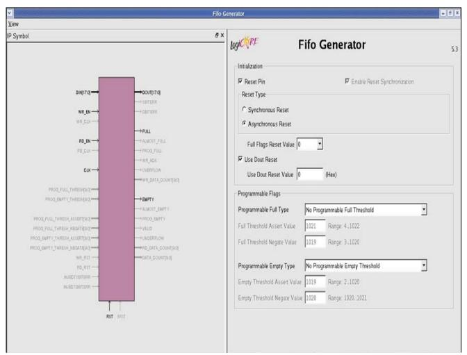
Figure 3-4: Programmable Flags and Reset Screen
