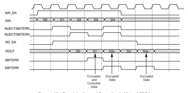
Figure 4-25: Error Injection and Correction in Virtex-6 FPGA
