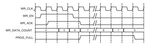
Figure 4-12: Programmable Full Single Threshold: Threshold Set to 7
