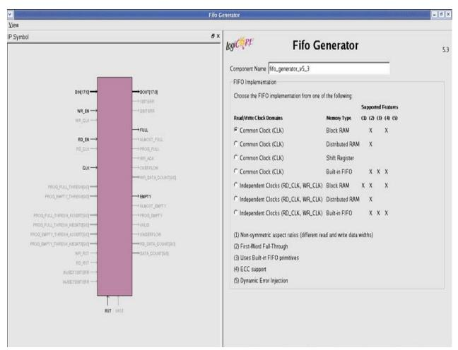
Figure 3-1: Main FIFO Generator Screen
