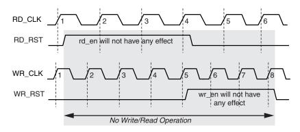
Figure 4-34: Synchronous Reset: FIFO with Independent Clock - RD\_RST then WR\_RST
