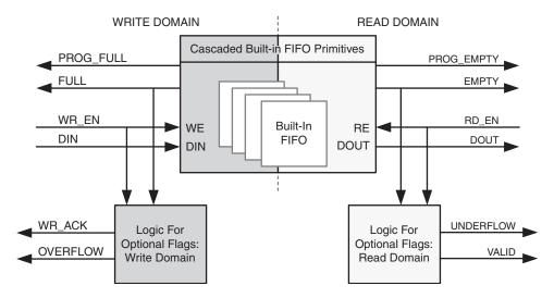
Figure 4-3: Functional Implementation of Built-in FIFO
