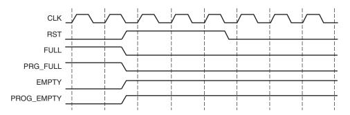
Figure 4-29: Built-in FIFO, Asynchronous Reset Behavior
