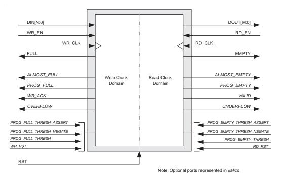
Figure 4-1: FIFO with Independent Clocks: Write and Read Clock Domains
