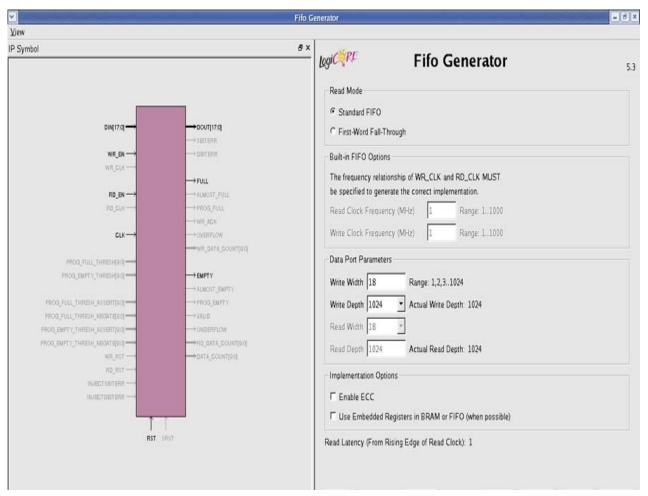
Figure 3-2: Performance Options and Data Port Parameters Screen
