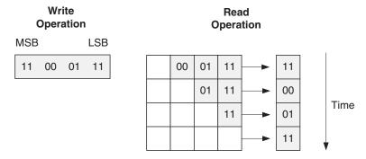
Figure 4-19: 4:1 Aspect Ratio: Data Ordering
