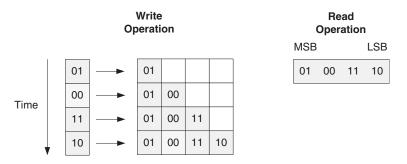
Figure 4-17: 1:4 Aspect Ratio: Data Ordering
