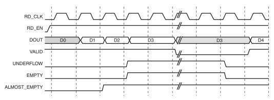
Figure 4-22: FWFT Read Operation for a Synchronous Built-in FIFO with User Embedded Registers Enabled
