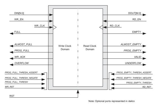
Figure 2-1: FIFO with Independent Clocks: Interface Signals
