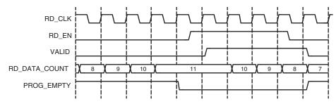
Figure 4-15: Programmable Empty with Assert and Negate Thresholds:
