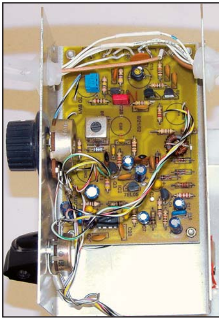
Figure 5 —This version of the receiver uses the FAR Circuits PC board and a RadioShack 270-238 aluminum box. Because the box is a bit wide for most hands, this version is easier to use when mounted on a wooden handle. The SENSE switch is a doorbell button easily operated with the index finger, and the RF GAIN and TUNING controls are easily reached with the other hand. (Left-handed ARDFers would probably want to move the controls to the other side of the box.) Note the orange tape on the loop, indicating the sense antenna null as described in the text.
